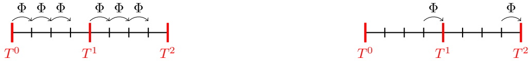
(a) F-relaxation is the parallelized application of \Phi , the time integration operator, to each of the F-points.
